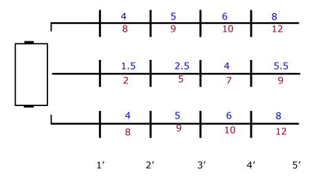
Offset voltage and discharge time determined using charged plate monitor. Discharge times are in seconds from 1000V to 100 V
