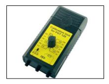
The PGT130.DT.CU periodic verification unit is used to check that the PGT120 tester is working properly.
