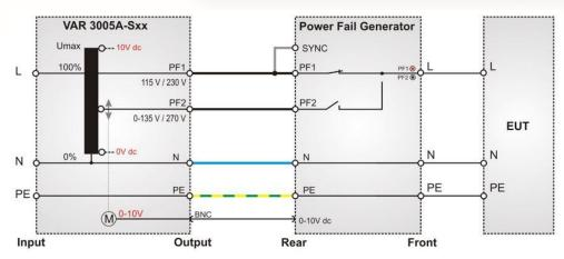
**Voltage interruptions (DIPS)** will cause a reduction of the power supply voltage for a certain period of time, three different test levels are required in IEC/EN 61000-4-11:
