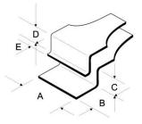
**Tip Dimensions:** (tip thickness) 0.35 mm - 0.014 inch
