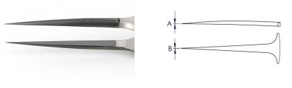
**Tip Dimensions:** A (tip thickness) 0.07 mm - 0.003 inch B (tip width) 0.12 mm - 0.005 inch
