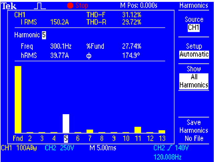
Conduct harmonic distortion measurements with TPS2PWR1 software.
