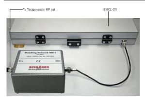
The matching network CDN EMCL-NW\_10 is not required for the EMCL-35.
