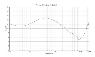
Measured amplifier power to achieve the highest level required in EN 61000-4-6 of 10 V. Measurement was carried out with 6 dB attenuator and 80% amplitude modulation.
