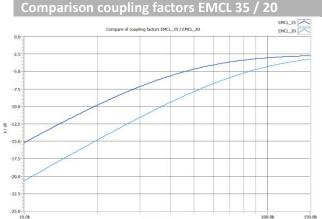
The high coupling factor of the EMCL-35 allows a test according to level 3 (10V) of IEC 61000-4-6 already at 10 kHz with the test generator CDG 7000-75-10.
