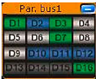
The signal activity of the digital channels is displayed in the signal icon independently of the oscilloscope settings.
