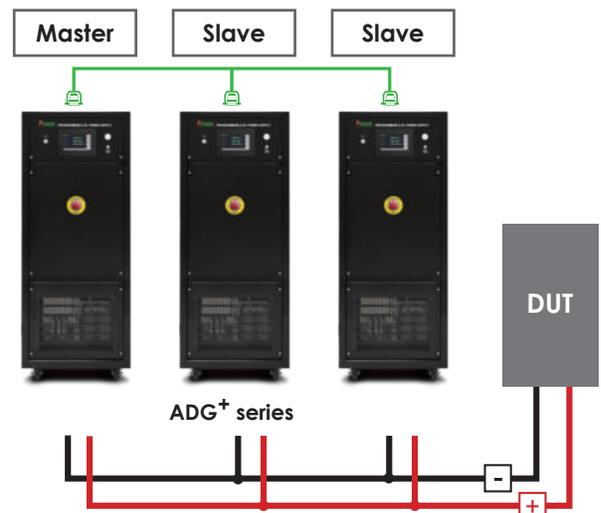
The output power of the ADG+ series is up to 300kW per unit, which can be expanded to 1800kW through simple master-slave operation (max. 5 units). User can simply operate the master unit, the slave unit will receive and reply the data accordingly and equally share the load current. ADG+ series is one of the few high-power DC power supply with parallel feature on the market. The availability for single-unit and parallel operation provides greater flexibility for application.
