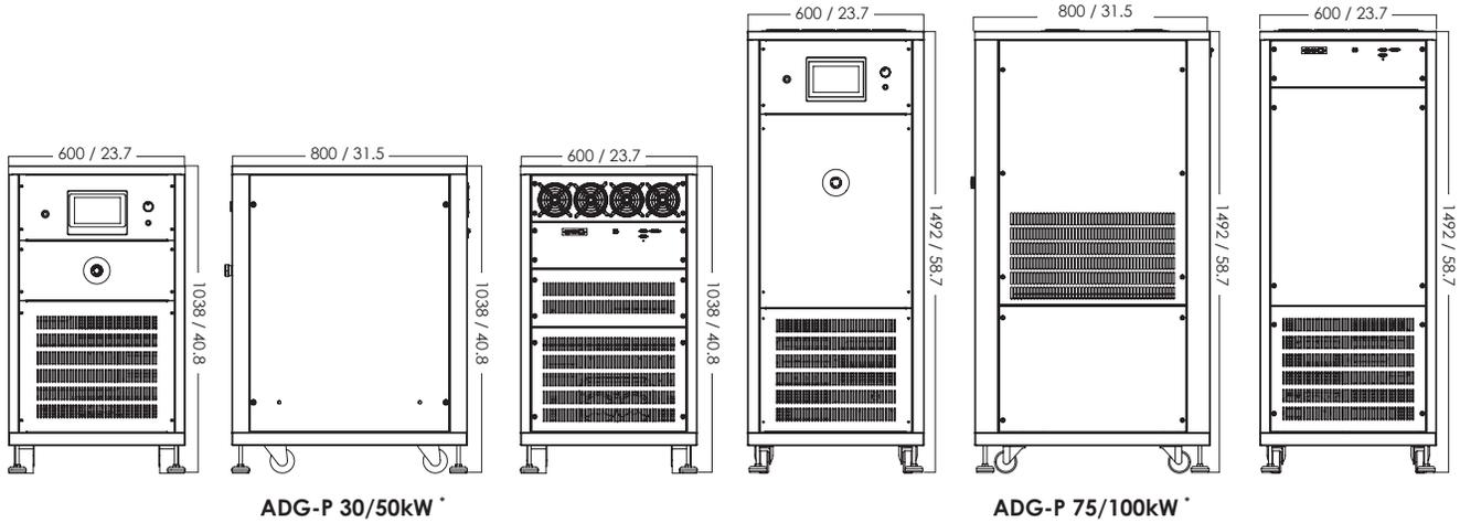
\* The diagrams and dimensions are for 380V input models.
