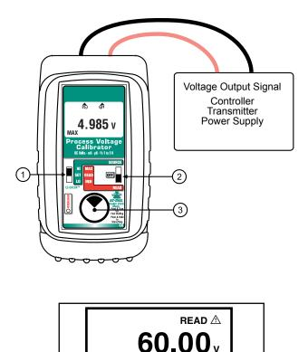
Signals exceeding  $\pm 60.00$  VDC are indicated by  $\triangle$  on the display.
