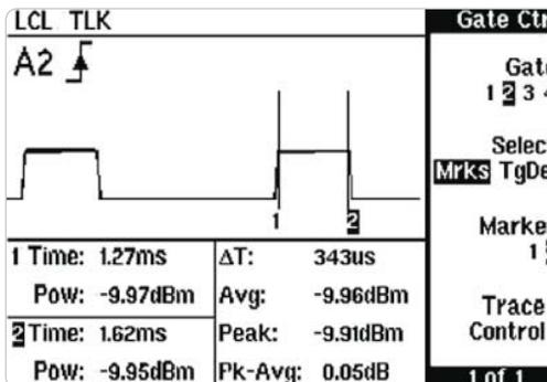
Figure 12. Average and peak power of second pulse
