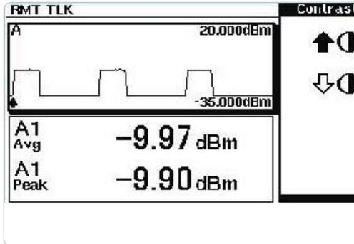
Figure 11. The Bluetooth signal is shown in the upper window. Average and peak power in a single Bluetooth DH1 data burst appear in the lower window.
