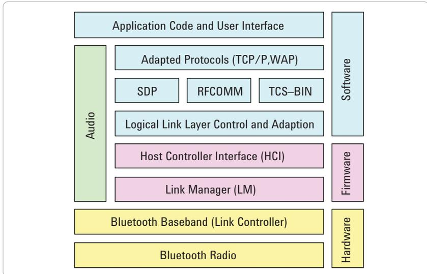
Figure 2. The Bluetooth protocol stack
