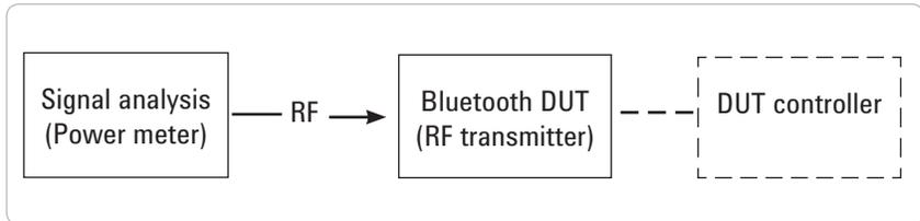
Figure 3. Test setup for a Bluetooth transmitter with power meter
