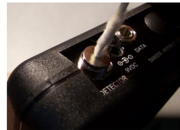
5 Using as little pressure as possible, rotate the cotton toothpick tip in the detector port to clear away any dust or dirt that has accumulated on the detector.
