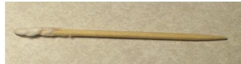
2 Wet the cotton toothpick tip with the isopropyl alcohol.
