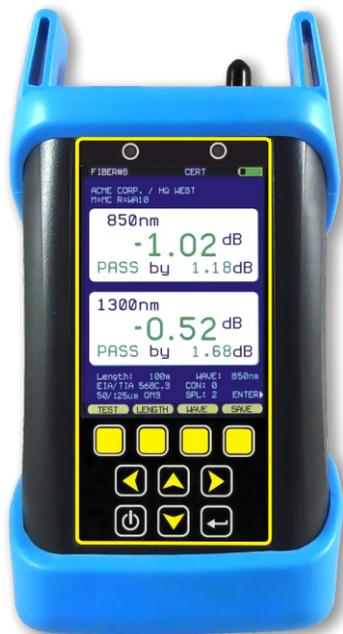
The **Fiber OWL 7** is a highly accurate hand-held optical power meter, capable of performing a wide range of functions from simple optical power and loss measurements to full-featured standards-based link certification (when used with a WaveSource Pro light source\*).
