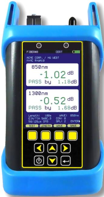
The Fiber OWL 7X is a highly accurate hand-held optical power meter, capable of performing a wide range of functions from simple optical power and loss measurements to full-featured standards-based link certification (when used with a WaveSource Pro light source\*).
