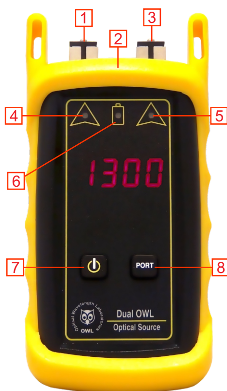
Figure 1 - Dual OWL Multimode Light Source
