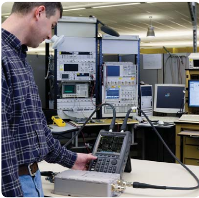
Tower mounted amplifier (TMA) measurement
