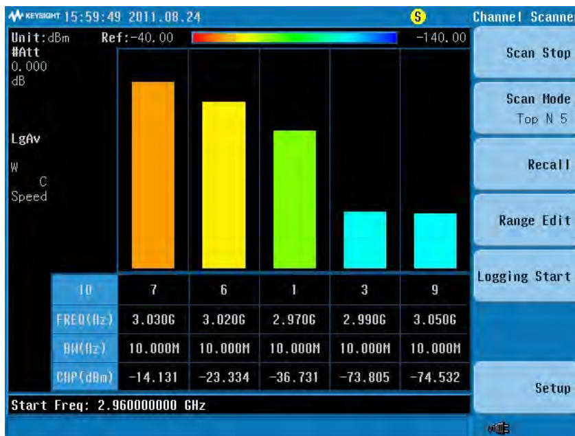
HSA Channel scanner option allows the user to easily measure channel power of multiple channels and export data for mapping applications like Google Earth and MapInfo
