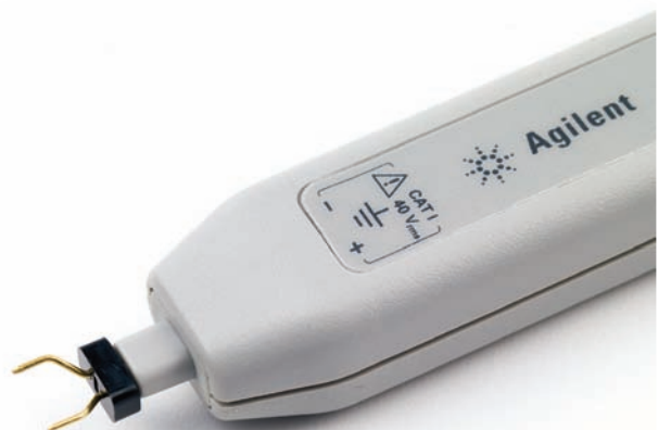
Figure 17. The variable pitch spacing adapter that fits over the N2793A/N2819A allows you to probe two adjacent IC leads or test points easily.
