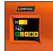
Tip temperature displayed on large color screen.
