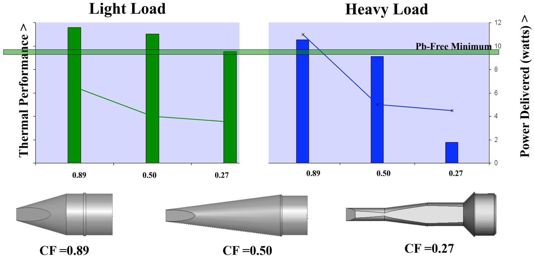
**Conductivity Factor = Energy Transfer Capability of the Tip Geometry
