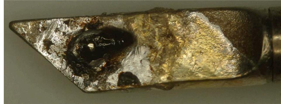
To eliminate this risk, **NEVER** feed the solder wire into the soldering tip. The solder wire should be fed onto the component and/or terminal
