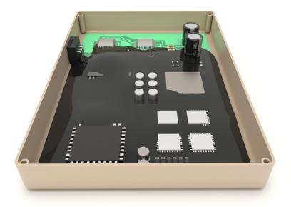
MG Chemicals has a series of high-quality potting compounds and encapsulation resins for the electronics industry. They add mechanical strength to assembly housings, fill large voids, insulate components from static discharge, and protect against exposure to chemicals, humidity, and salt water.
