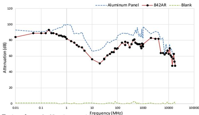
Test performed with a two-coat thickness.
