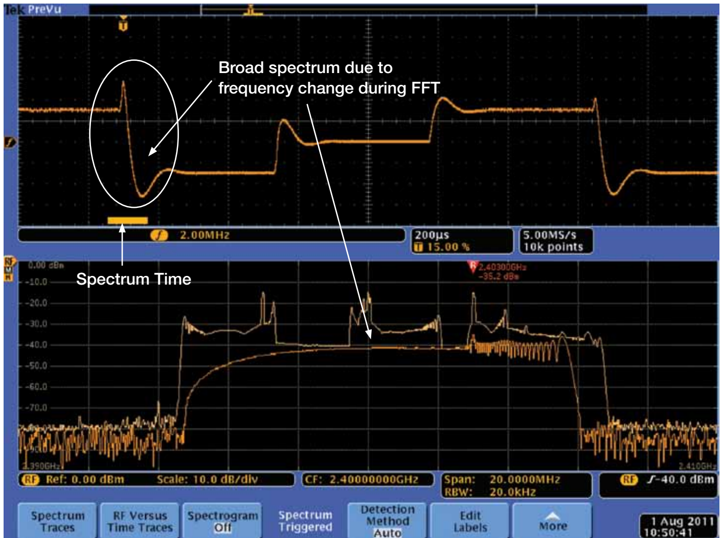
Figure 31. Broad spectral energy of signal is displayed during frequency transition.
