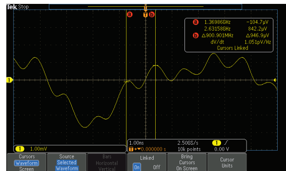
Figure 14: Cursor measurements identify noise as 900 MHz
