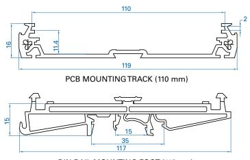
DIN RAIL MOUNTING FOOT (110mm)
