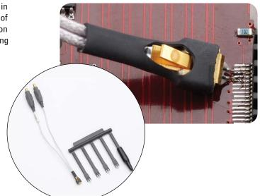
N5444A 2.92 mm/3.5 mm/SMA probe head (28 GHz) allows you to connect two 2.92 mm, 3.5 mm or SMA cables to make a differential measurement on a single oscilloscope channel. Order N5448A 2.92 mm head flex cables (10" or 25 cm) to extend the cable length and add convenience.
