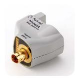
N5449A high impedance adapter allows the connection of probes that require a high impedance scope input such as a high impedance passive probe, 1147A current probe, or N2790A differential probe to the Infiniium 90000-X Series oscilloscopes. The N5449A provides switchable AC/DC coupling as well as 10:1 and 1:1 attenuation settings. The adapter comes with a N2873A 500 MHz 10:1 passive probe.
