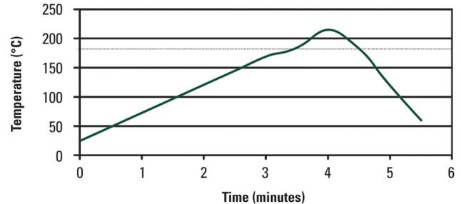
The profile shown here is designed for **Indium6.3** with Sn63/Pb37 and Sn62/Pb36/Ag2 under both air and nitrogen reflow atmosphere. It serves as a general guideline in establishing a reflow profile for these alloys.
