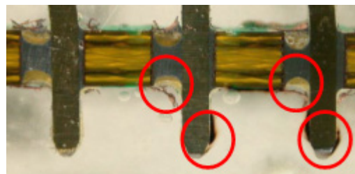
Solder starvation in PIP processed solder joint. Also note the excess residual flux.
