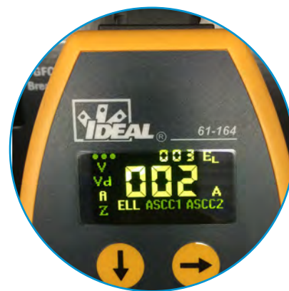
Estimated Load on Line in Amps
