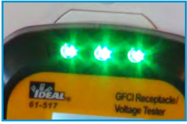
Green Lights Indicate Correct Wiring
