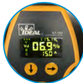
Displays Voltage Drop at 12, 15 & 20 Amps
