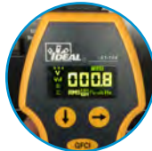
Displays neutral to ground voltage
