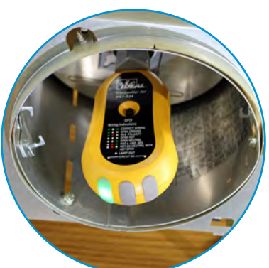
Lead Adapter Kit Provides adapters for use in lighting fixtures.
