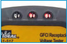
Red Lights Indicate Incorrect Wiring
