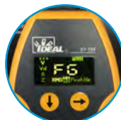
Detects and Displays false or "bootleg" ground
