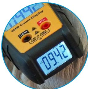
**Patented TightSight® Backlit Display** eliminates need to bend or twist conductors or place your head near or in the panel and allows you to easily read the bottom display when taking all measurements.
