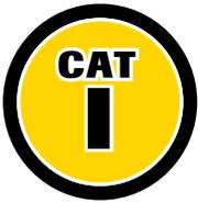
**Category I** – The signal level for telecommunications, electronic and other low-energy equipment with transient limiting protection. Peak impulse transient range is 600-4,000 volts with 30 ohm source.
