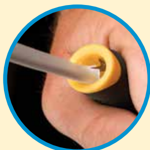
Insert wire into specially designed blade.
