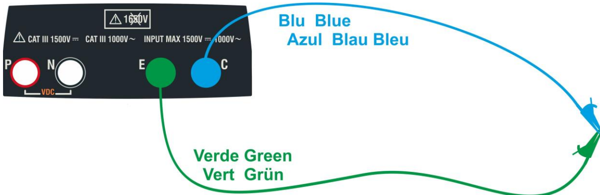
Fig. 4: Compensation of the measuring cables resistance
