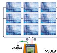
INSULATION **MEASUREMENT IN "FULL PV FIELD**" MODE
