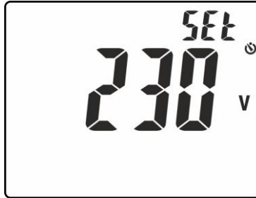
Fig. 6: Setting the rated voltage in Loop measurement
