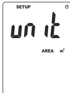
Fig. 3: Setting the measuring unit of the area of the duct
