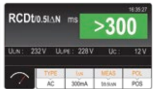
Test on RCDs
