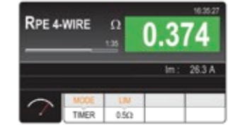
4-wire continuity test
