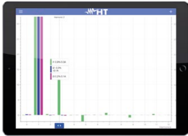
Current and voltage harmonics.
