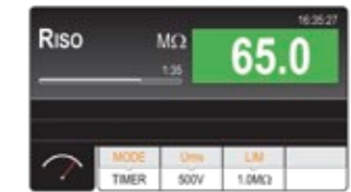
Measurement of insulation resistance
