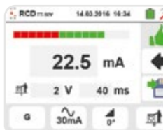
Result of ramp test on RCD.
