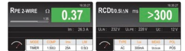
2-wire continuity test
