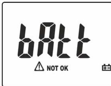
Fig. 45: Low battery indications
