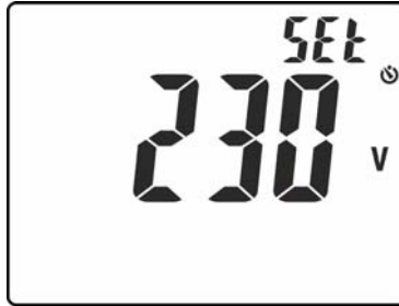
Fig. 6: Setting the rated voltage in Loop measurement
