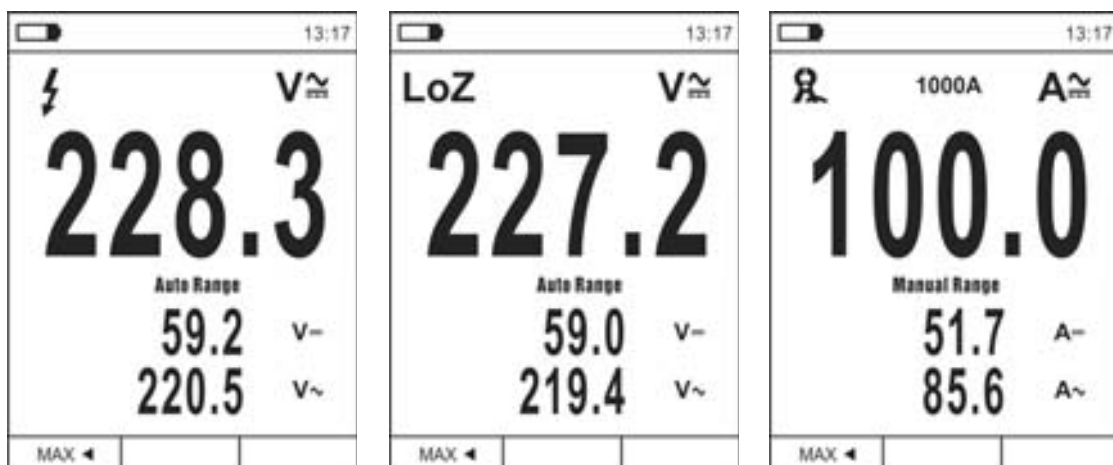
Fig. 6: Description of AC+DC Voltage and Current measurement
