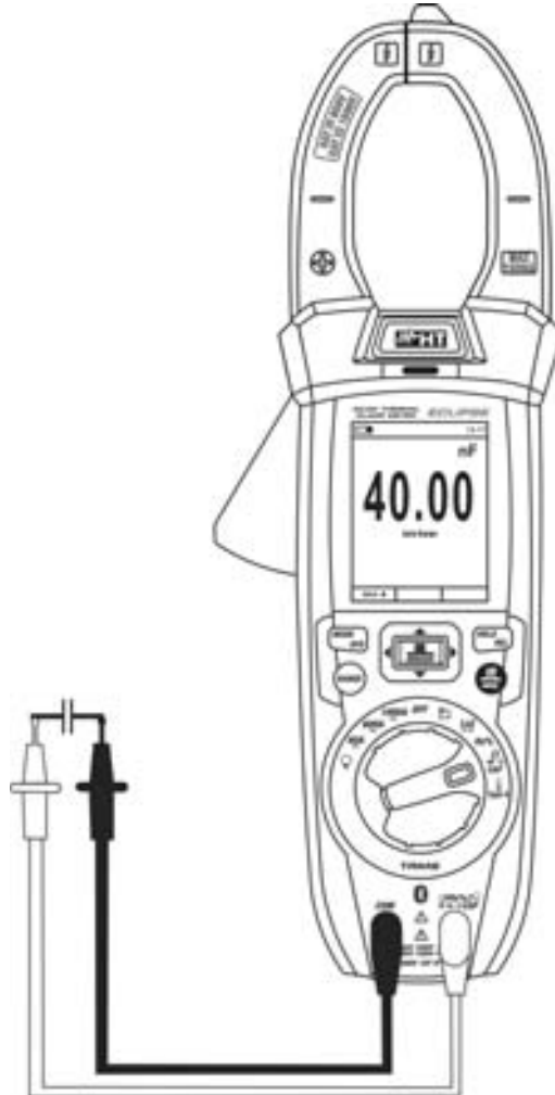
Fig. 29: Use of the instrument for Capacitance measurement
