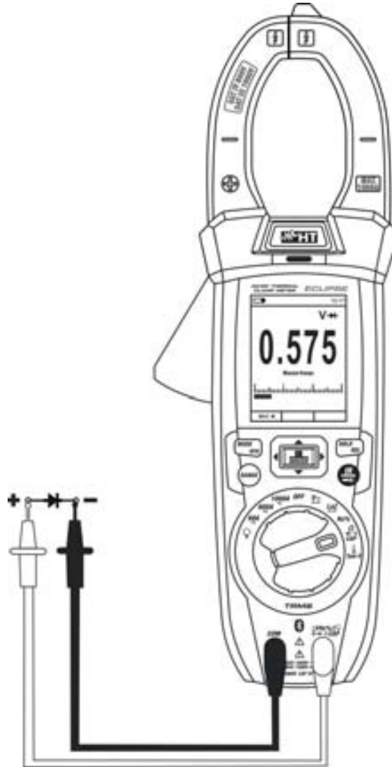
Fig. 28: Use of the instrument for diode test
