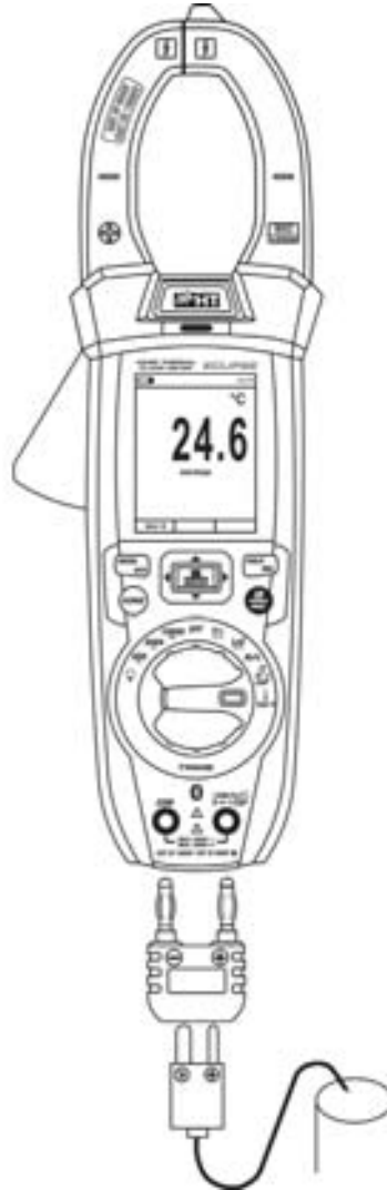
Fig. 30: Use of the instrument for Temperature measurement
