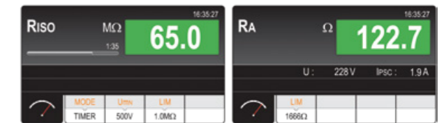
Measurement of insulation resistance
