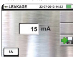
Measurement of leakage current with optional clamp HT96U.
