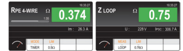
4-wire continuity test
