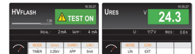
Dielectric strength test
