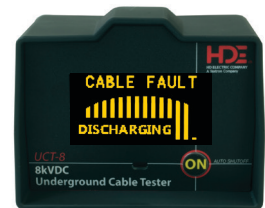
Faulted cable test results - cable discharging
