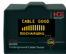
Good cable test results - cable discharging
