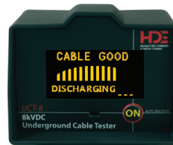
Good cable test results - cable discharging
