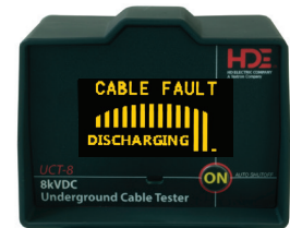
Faulted cable test results - cable discharging
