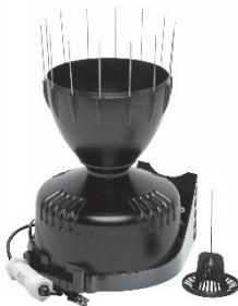
The Davis (0.01" or 0.2 mm) Rain Gauge smart sensor is designed to work with HOBO® stations. The smart sensor has a plug-in modular connector that allows it to be added easily to a HOBO station. All sensor parameters are stored inside the smart sensor, which automatically communicates configuration information to the logger without the need for any programming or extensive user setup. **Note:** This sensor has been modified to work with Onset station loggers only.
