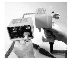
3) Touch the Transmitter and Receiver probes to each other. Red lights on both units indicate they are working properly.
