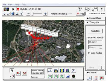
Locate interference with integrated mapping solution and triangulate multiple measurements with resulting areas of uncertainty
