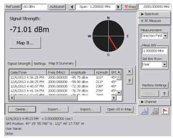
Use Direction Finding display - use compatible antennas and field strength measurements to find the likely directions to signals of interest. Results can be sent to the Mapping application for further geolocation analysis.
