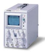
The GOS-310, 10MHz analog oscilloscope is designed for education, hobby and maintenance use. The GOS-310 is applicable for various market fields with a sensitivity of 5mV/div, internal and external triggering and a number of triggering modes (Auto, Norm, Ext and TV sync.). A 10MHz bandwidth, single channel operation, a light 4.6kg weight and a compact design make the GOS-310 the best choice for an affordable analog oscilloscope with effective performance.
