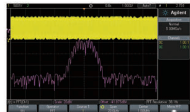
KEYSIGHT DSOX2000A - FFT Display
