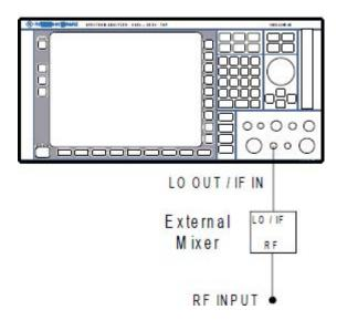
1. 1. Connect the LO OUT / IF IN output of the R&S FSV to the LO/IF port of the external mixer. The nominal LO level is 15.5 dBm.
