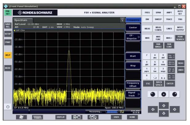
Using the F6 key you can toggle the Front Panel display on and off.
