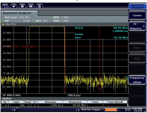
Fig. 6-13: Display of the filter edge of the 300 kHz filter as an FM discriminator characteristic
