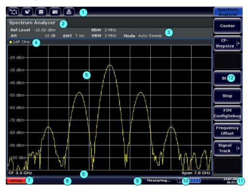
Fig. 5-1: Screen layout of the R&S FSV during analyzer operation
