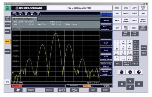
You can operate all keys and softkeys using the mouse. The rotary knob is simulated using the knob buttons.
