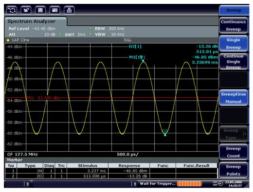
Fig. 6-14: Demodulated FM signal
