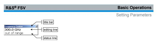
Fig. 5-2: Edit dialog box for parameter entry
