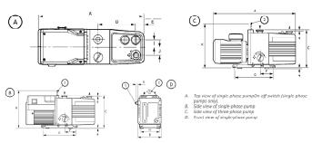
A. Lifting bracket (RVR and RV12 pumps only: a lifting handle is fitted to the RV3 and RV5 pumps).
