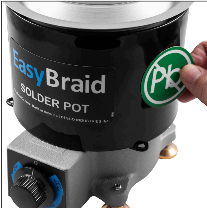
Figure 3. Applying the lead-free label onto the Solder Pot
