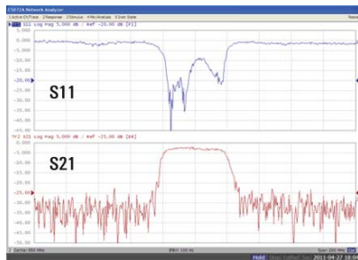
Figure 7. Accurate measurements with low signal input, Upper (power = -55 dBm with external 20 dB attenuator), Lower (power = -75 dBm with built-in attenuator)
