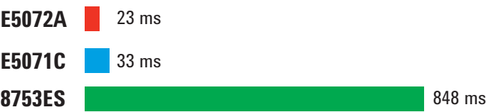
Figure 15. Measurement speed comparison: 1601 points, full 2-port cal, 1 GHz to 1.2 GHz IFBW = 6 kHz (8753ES), 500 kHz (E5071C and E5072A)
